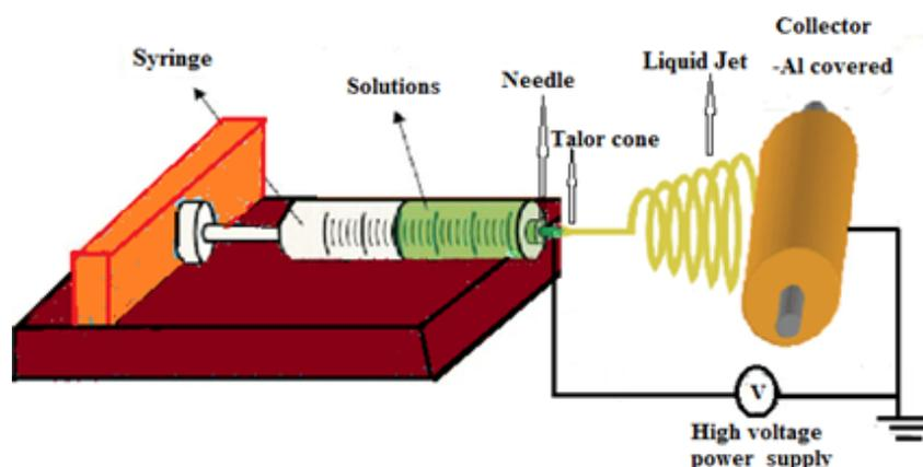
**Scheme 1.** Schematic of a typical electrospinning setup
