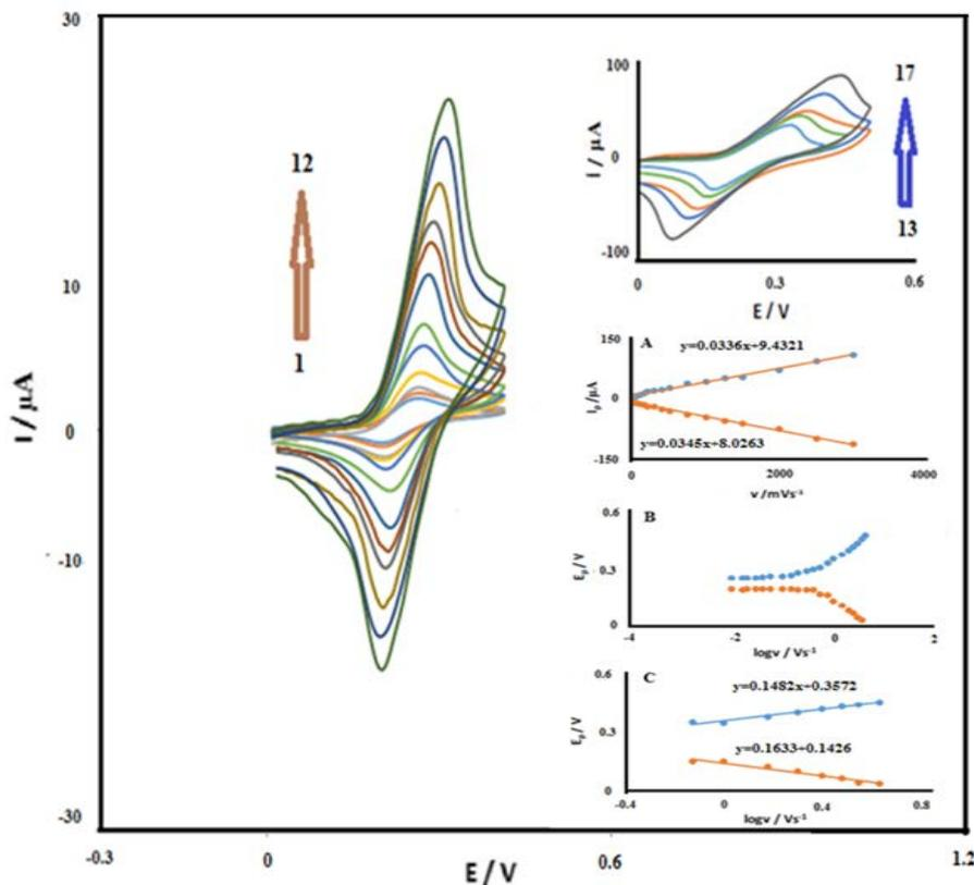
**Fig. 2.** Cyclic voltammograms of DMC/NF/CP in 0.1 M phosphate buffer (pH 7.0) at scan rates: (1) 10, (2) 20, (3) 30, (4) 40, (5) 50, (6) 100, (7) 150, (8) 200, (9) 300, (10) 400, (11) 500, (12) 750, (13) 1000, (14) 1250, (15) 1500, (16) 2000, and (17) 2500  $\text{mVs}^{-1}$ . Insets: (A) Variation of peak currents with sweep rate. (B) Variation of  $E_p$  vs. the logarithm of the scan rate. (C) Magnification of the same plot for high scan rates
