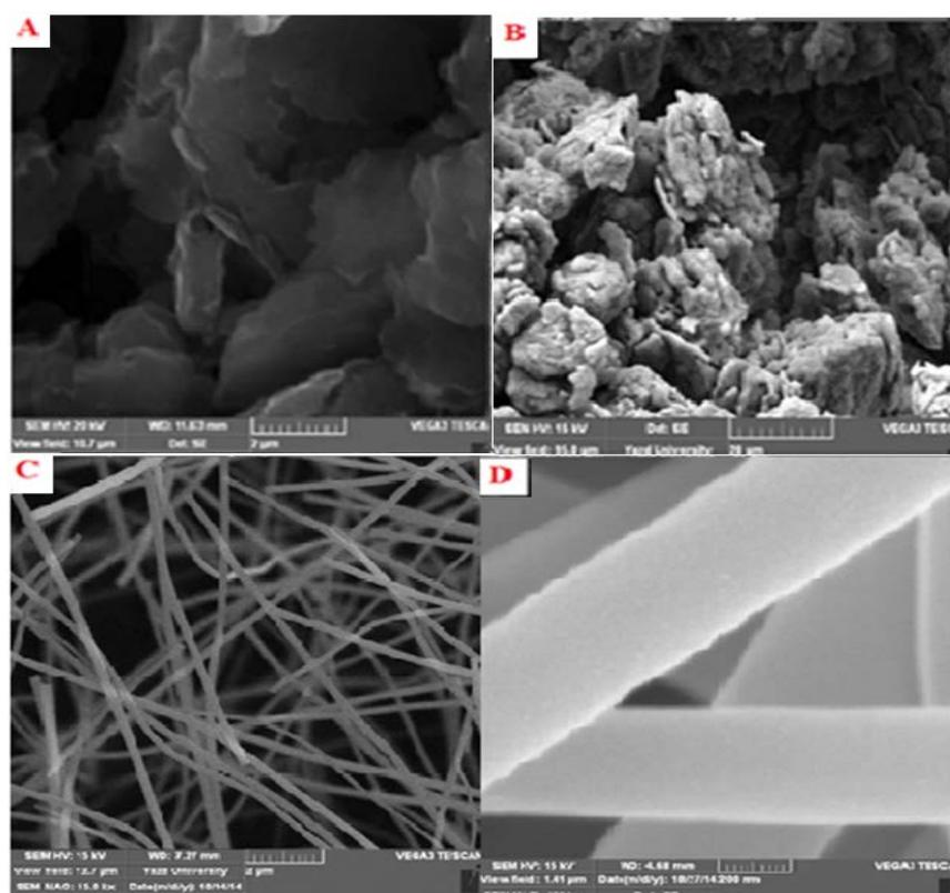
**Fig. 1.** SEM images of different carbon paste electrodes. CPE (A), CPE-NF (B), calcinated TiO<sub>2</sub> nanofibers (600 °C) (C), TiO<sub>2</sub> nanofiber with large magnification (D)
