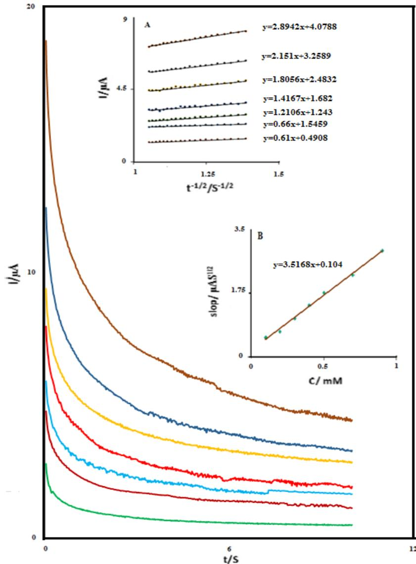
**Fig. 6.** (A) Chronoamperometric response of DMC/NF/CP in 0.1M phosphate buffer solution (pH 7.0) at potential step of 300 mV for different concentration of Trp.. The numbers of 1–7 correspond to 0.1, 0.2, 0.3, 0.4, 0.5, 0.6 and 0.7 mM Trp.. Insets: (A) Plots of  $I$  vs.  $t^{-1/2}$  obtained from the chronoamperograms 1–7 and (B) plot of the slopes of the straight lines against the Trp. Concentration
