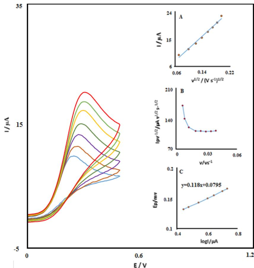
**Fig. 5.** CVs DMC//NF/CP in 0.1 M phosphate buffered solution (pH 7.0) containing 0.3 mM Trp. at various scan rates, from inner to outer scan rates of 5, 10, 15, 20, 25, 30, and 40  $\text{mV s}^{-1}$ , respectively. Insets: variation of (A) anodic peak current versus  $v^{1/2}$ ; (B) normalized current ( $I_p/v^{1/2}$ ) versus  $v$ ; (C) Tafel plot derived from the rising part of voltammogram recorded at a scan rate of 10  $\text{mV s}^{-1}$
