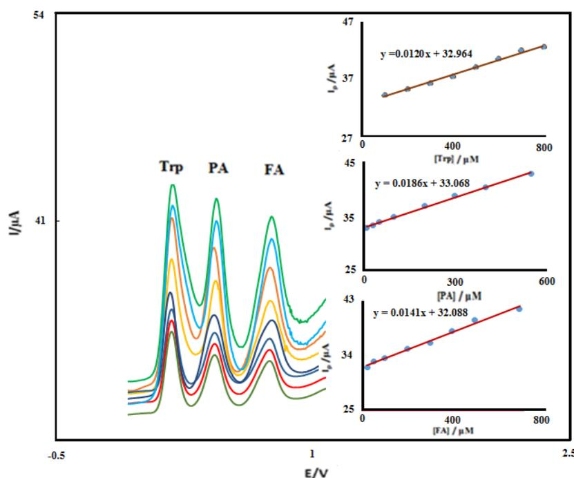
**Fig. 8.** DPVs of DMC/NF/CP in 0.1 M phosphate buffer solution (pH 7.0) containing different concentrations of Trp.+PA+FA in  $\mu\text{M}$  (from inner to outer): mixed solutions of 20.0+10.0+20.0, 70.0+30.0+50.0, 120.0+50.0+100.0, 250.0+100.0+200.0, 350.0+200.0+300.0, 450.0+300.0+400.0, 550.0+400.0+500.0 and 750.0+550.0+700.0, respectively. Insets: (A–C) plots of the peak currents as a function of Trp., PA and FA concentration, respectively
