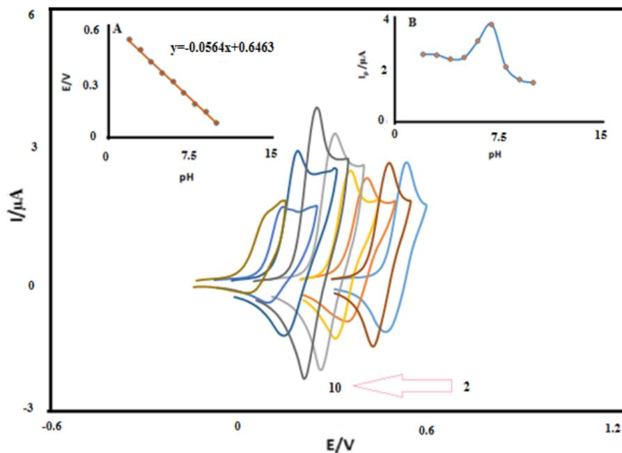
**Fig. 3.** CVs of DMC/NF/CP in different pH values of 2-10 the insets A and B, show effects of pH on the anodic peak potential and anodic peak current in phosphate buffer solution Scan rate  $50 \text{ mV s}^{-1}$
