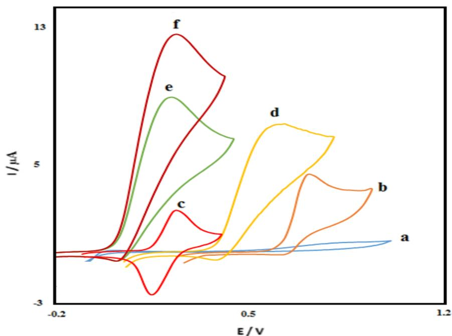
**Fig. 4.** CVs of (a) unmodified CPE in 0.1 M phosphate-buffered solution (pH 7.0) at scan rate of  $15 \text{ mVs}^{-1}$ ; (b) as (a)+0.3 mM Trp.; (c) as (a) at the surface of DMC/NF/CP; (d) as (b) at the surface of NF/CP; (e) as (b) at the surface of DMC/CP, (f) as (b) at the surface of DMC/NF/CP
