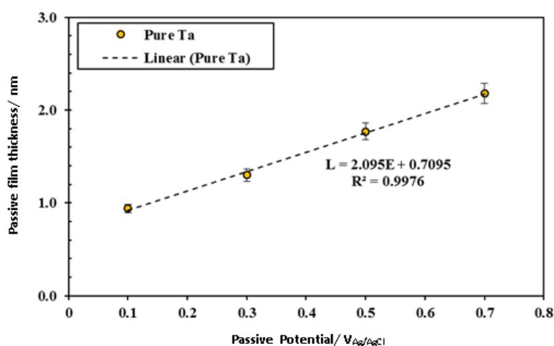
**Fig. 6.** Role of passive potential on the calculated passive film thickness of pure Ta in 0.1 M H<sub>2</sub>SO<sub>4</sub> solution
