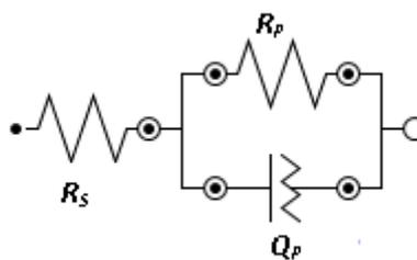
**Fig. 4.** The Randles circuit for the modeling experimental EIS data [19]
