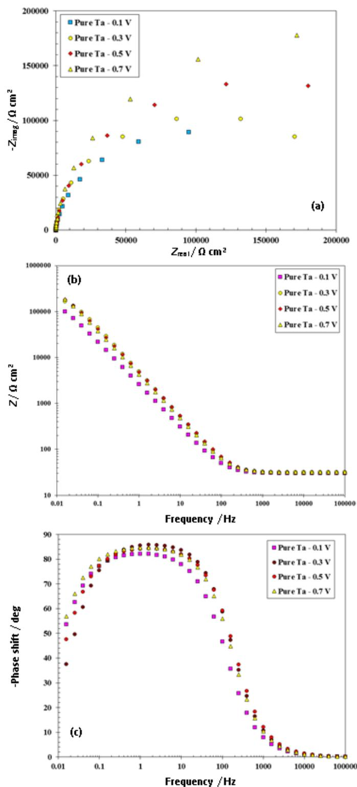
**Fig. 3.** Role of passive potential on the (a) Nyquist, (b) Bode, and (c) Bode-phase plots of pure Ta in 0.1 M  $\text{H}_2\text{SO}_4$  solution
