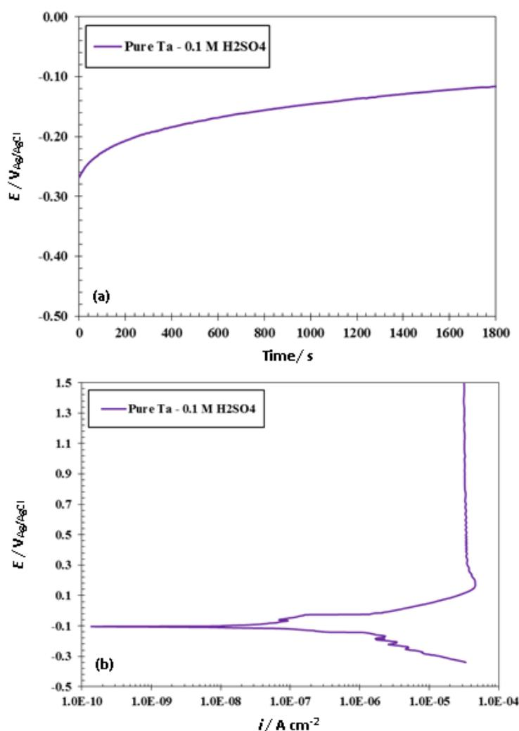
**Fig. 1.** (a) OCP and (b) PDP plot of pure Ta sample in 0.1 M H<sub>2</sub>SO<sub>4</sub> solution
