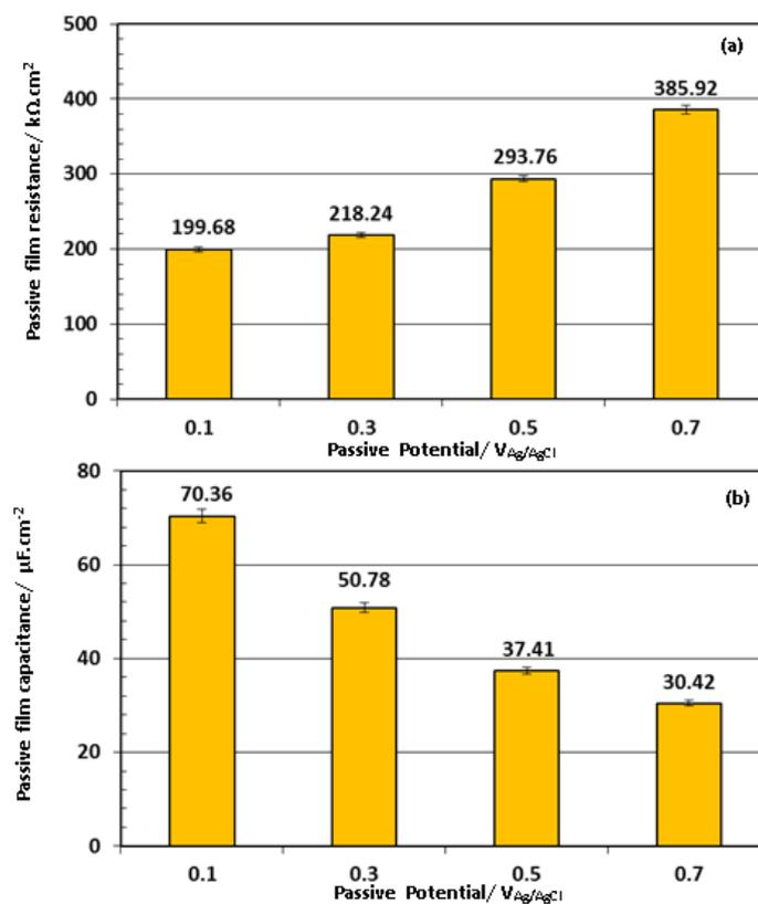
**Fig. 5.** Effect of passive potential on the (a) passive film resistance and (b) passive film capacitance of pure Ta in 0.1 M H<sub>2</sub>SO<sub>4</sub> solution
