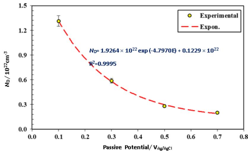
**Fig. 9.** Role of anodic passive potential on the calculated donor density of the passive layers formed on pure Ta in 0.1 M H<sub>2</sub>SO<sub>4</sub> solution
