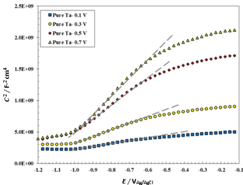
**Fig. 7.** Role of passive potential on the M–S plots of pure Ta in 0.1 M  $H_2SO_4$  solution
