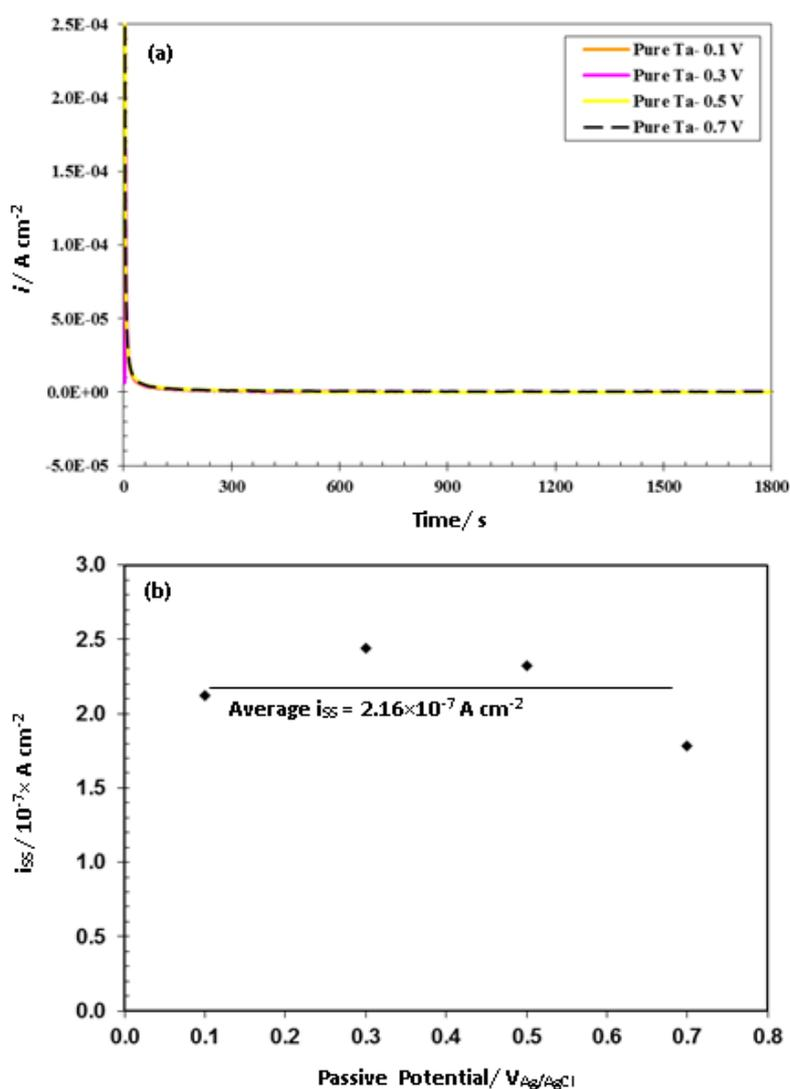
**Fig. 2.** (a) Potentiostatic polarization plots of pure Ta in 0.1 M H<sub>2</sub>SO<sub>4</sub> solution, and (b) steady-state passive current density obtained during the potentiostatic growth of the passive layers
