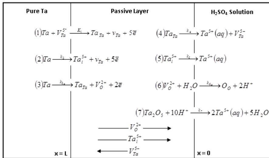
**Fig. 8.** The modified PDM for passivation of Ta in 0.1 M H<sub>2</sub>SO<sub>4</sub> solution.  $V_{Ta}^{5-}$ =Ta vacancy on the Ta sublattice of the passive layer,  $Ta_i^{5+}$ =interstitial Ta,  $Ta_{Ta}$ =Ta cation on the Ta sublattice of the passive layer,  $V_O^{2+}$ =oxygen vacancy on the oxygen sublattice of the passive layer,  $O_O$ =oxygen anion on the oxygen sublattice of the passive layer,  $Ta^{5+}(aq)$ =Ta cation in solution
