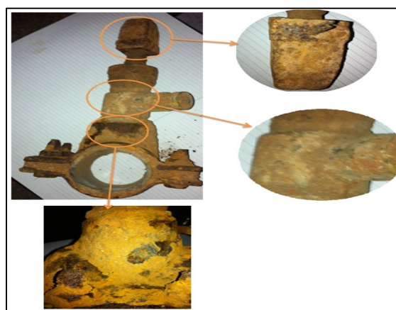
Fig. 1. Example of deterioration of support fittings which are suitable for connecting domestic service lines buried in the Azrou soil
