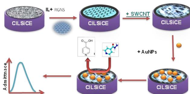
**Fig. 3.** Schematic of the sensor preparation
