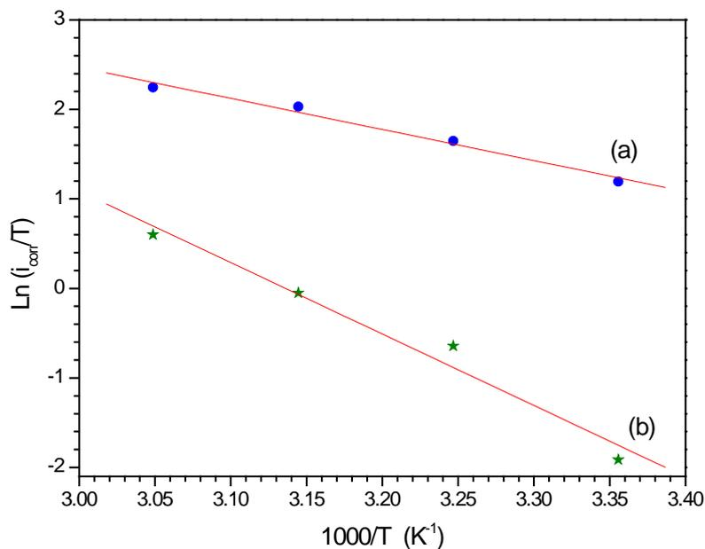
**Fig. 9.** Transition-state plots for carbon steel in 1.0 M HCl (a) without and (b) with 200 ppm of PS
