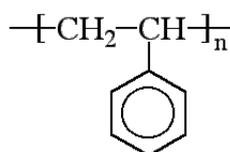
**Fig. 1.** Chemical structure of poly(1-phenylethene)
