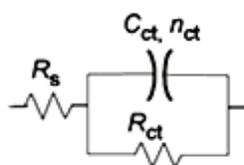
**Fig. 6.** Equivalent circuit used to model impedance data in 1.0 M HCl solutions in the presence of different concentration of PS
