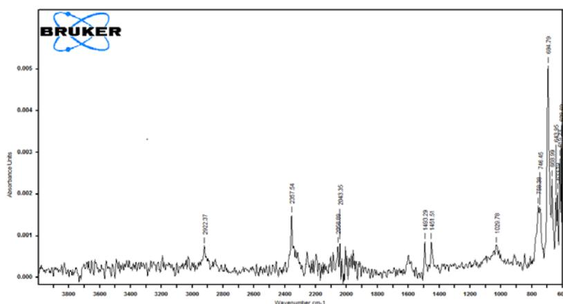
**Fig. 3.** FTIR spectra of Poly(1-phenylethene)
