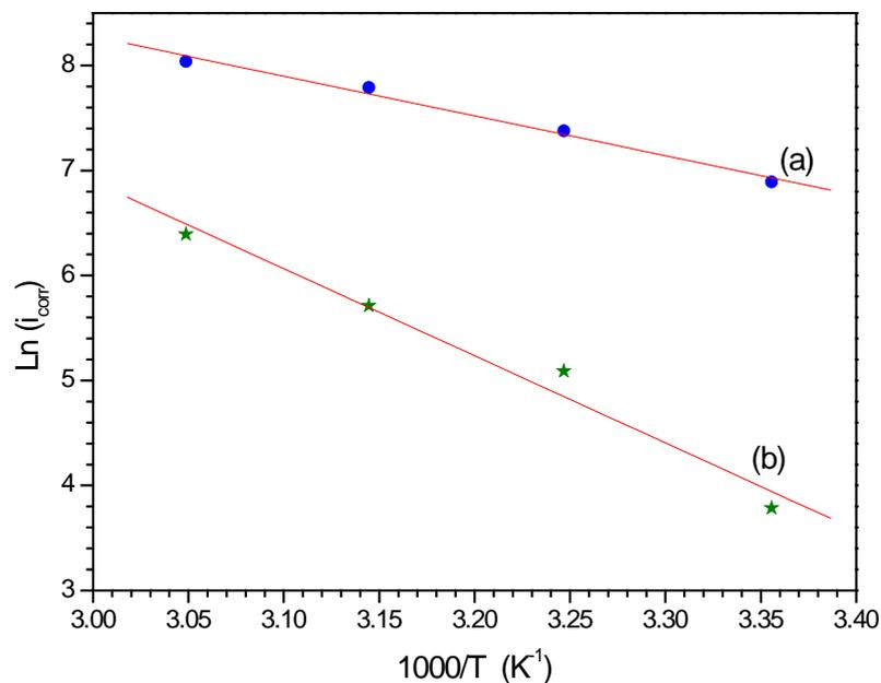
**Fig. 10.** Arrhenius plots of carbon steel in 1.0 M HCl (a) without and (b) with 200 ppm of PS
