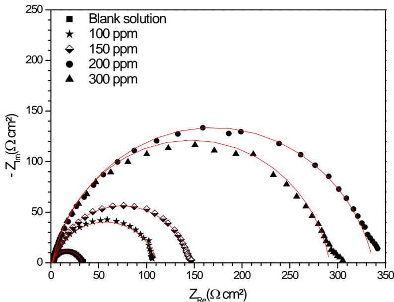
**Fig. 5.** Nyquist plots for carbon steel in 1.0 M HCl solution in the absence and presence of various concentrations of PS at  $E_{corr}$  ( $T=298$  K). Scatter: Experimental curves and Red line: Fitting curves
