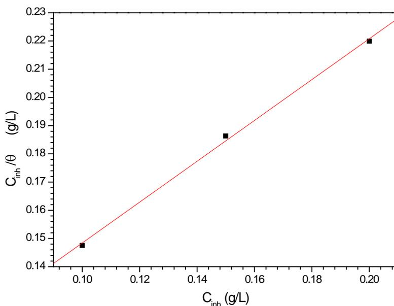
**Fig. 9.** Plot of the Langmuir adsorption isotherm of PS on the carbon steel surface at 298 K
