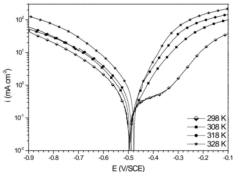
**Fig. 7.** Potentiodynamic polarization curves for carbon steel in 1.0 M HCl in the absence of PS at different temperature
