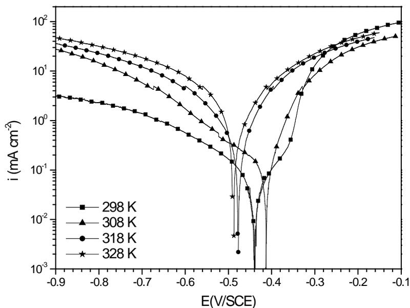
**Fig. 8.** Potentiodynamic polarization curves for carbon steel in 1.0 M HCl in the presence of 200 ppm of PS at different temperature
