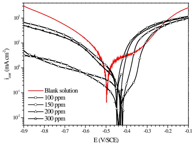
**Fig. 4.** Potentiodynamic polarization curves for carbon steel in 1.0 M HCl without and with different concentrations of PS
