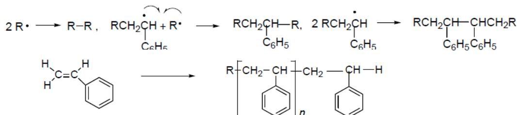
**Fig. 2.** Mechanism of polymerization of styrene
