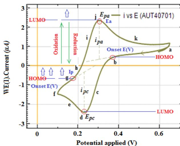
**Fig. 4.** Cyclic voltammogram of standard  $[\text{Fe}(\text{CN})_6]^{3+}$ : Graphical representation for the determination of onset potentials and HOMO-LUMO energy levels
