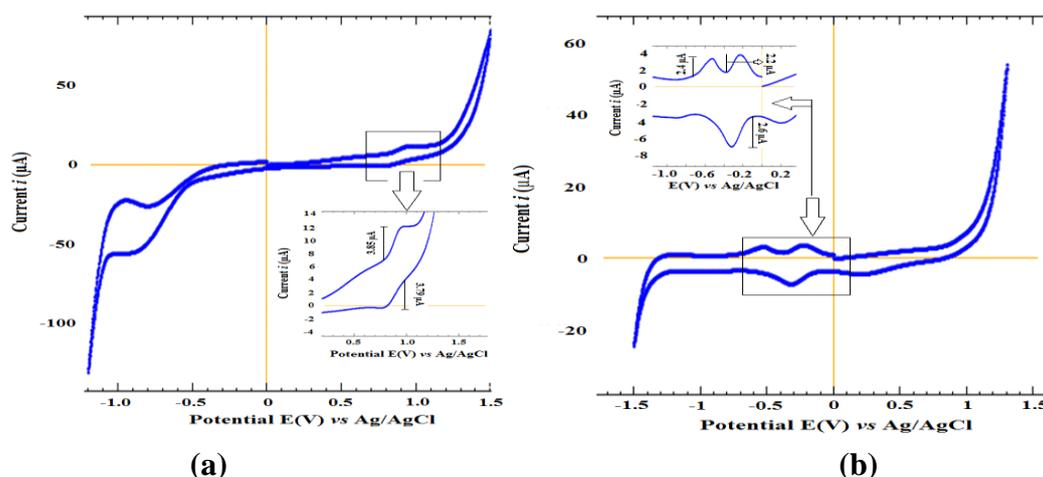
**Fig. 5.** Cyclic voltammograms of (a)  $[\text{Mn}^{\text{II}}\text{LCl}_2]$  and (b)  $[\text{Co}^{\text{II}}\text{LCl}_2]$  macrocyclic complexes in DMSO containing  $10^{-3}$  M of complex and 0.1 M TEAP as supporting electrolyte at a scan rate of  $200 \text{ mVs}^{-1}$ . The inserted voltammograms showed the onset potentials and enlarge of major redox couple
