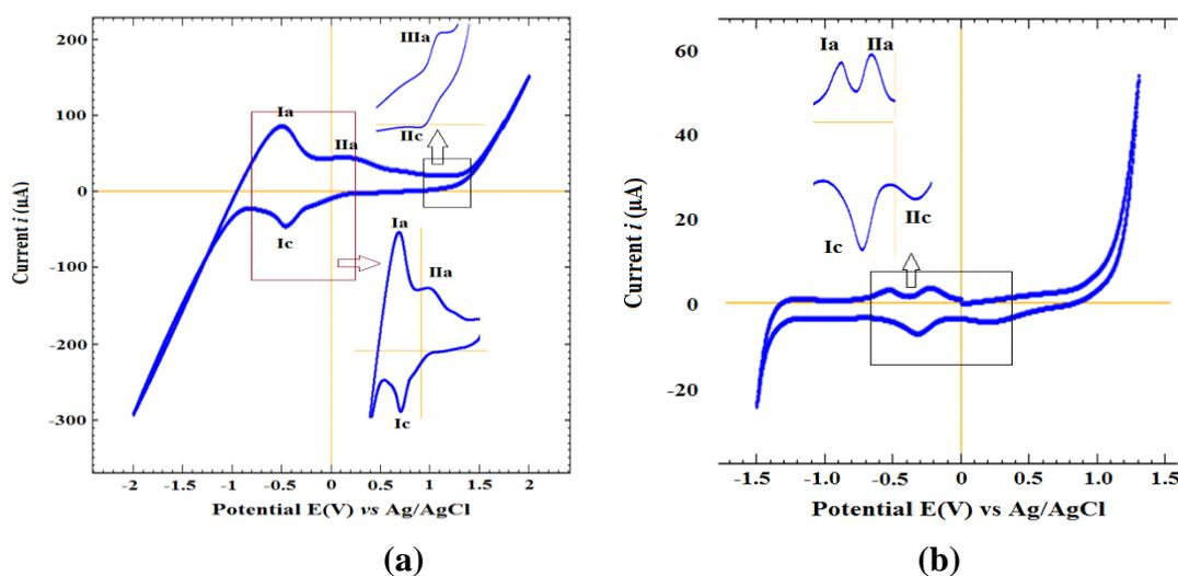
**Fig. 3.** Cyclic voltammograms of (a)  $[\text{Mn}^{\text{II}}\text{LCl}_2]$  and (b)  $[\text{Co}^{\text{II}}\text{LCl}_2]$  macrocyclic complexes in DMSO containing  $10^{-3}$  M of complex and 0.1 M TEAP as supporting electrolyte at a scan rate of 200 mV
