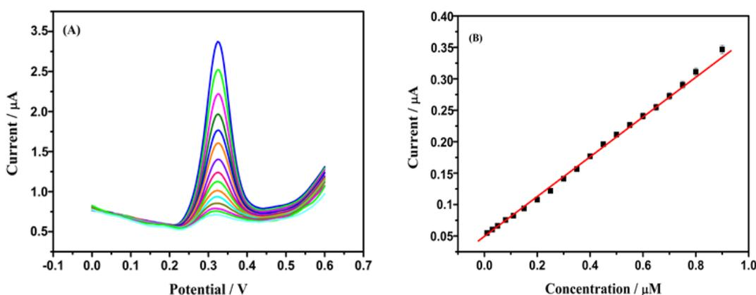
**Fig. 6.** (A) Illustrates the differential pulse voltammograms of acetaminophen at GMPGE in the range of  $1.0 \times 10^{-8} M$  to  $0.9 \times 10^{-6} M$  in phosphate buffer solution of pH 7.0; (B) Illustrates the relation between anodic peak current ( $i_{pa}$ ) vs. various concentration ( $C$ ) of acetaminophen in 0.1 M phosphate buffer solution of pH 7.0
