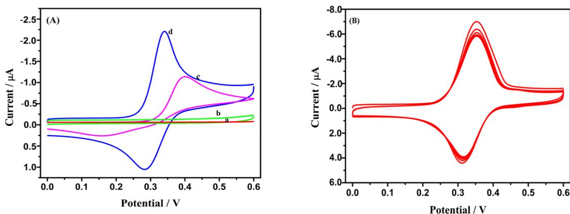
**Fig. 3.** (A) Depicts the cyclic voltammograms of phosphate buffer solution at PGE (a) and GMPGE (b), cyclic voltammograms obtained for 1mM acetaminophen at PGE (c) and GMPGE (d) in 0.1 M phosphate buffer solution of pH 7.0 at a scan rate of  $100 \text{ mV s}^{-1}$ ; (B) Depicts the successive voltammograms (10 cycles) of 1 mM acetaminophen at GMPGE in 0.1 M PBS of pH 7.0 at a scan rate of  $100 \text{ mV s}^{-1}$
