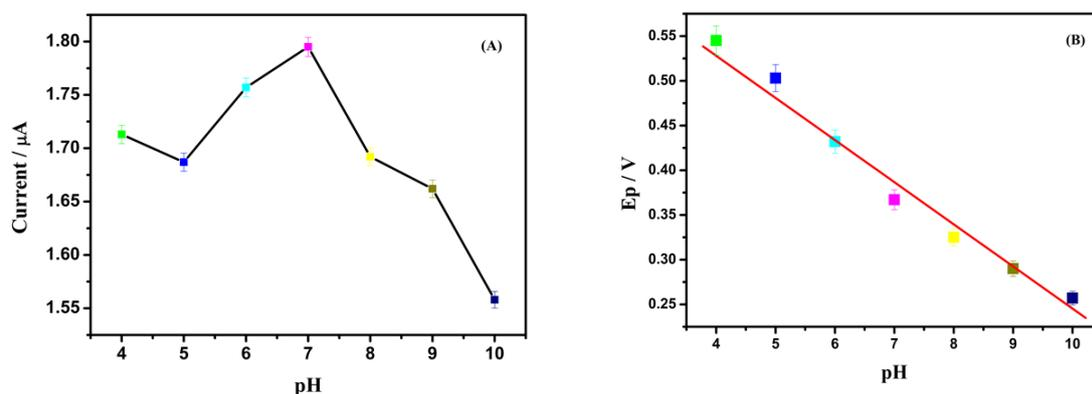
**Fig. 4.** (A) Illustrates the effect of pH (4.0, 5.0, 6.0, 7.0, 8.0, 9.0 and 10.0) on peak current of acetaminophen (20  $\mu$ M) at GMPGE in 0.1 M phosphate buffer solutions; (B) Illustrates the effect of pH on the peak potential of acetaminophen (20  $\mu$ M) at GMPGE in 0.1 M different phosphate buffer solutions
