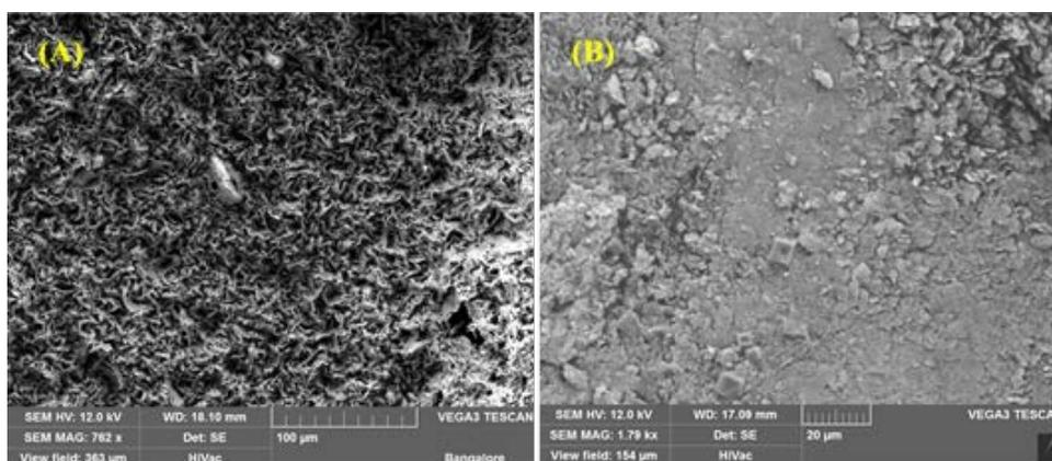
**Fig. 1.** Scanning electron microscopy images of (A) PGE and (B) GMPGE
