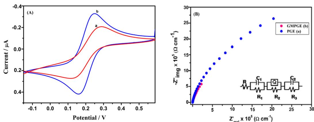
**Fig. 2.** (A) illustrates the cyclic voltammograms of 1 mM  $K_3[Fe(CN)_6]$  in 0.1 M KCl solution at PGE (a) and GMPGE (b) at a scan rate of  $100 \text{ mV s}^{-1}$ ; (B) EIS at PGE (a) at GMPGE (b) in 0.1 M KCl solution containing 1 mM  $K_3[Fe(CN)_6]$  solution with a frequency range: 10 kHz–0.1 Hz. Inset: Randle's equivalent circuit
