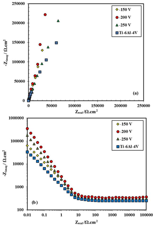
**Fig. 4.** (a) Nyquist, and (b) Bode curves Ti-6Al-4V samples coated under different bias voltages in SBF solution
