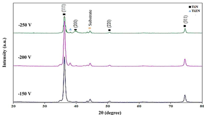
**Fig. 1.** XRD patterns of deposited coatings at different substrate bias voltages
