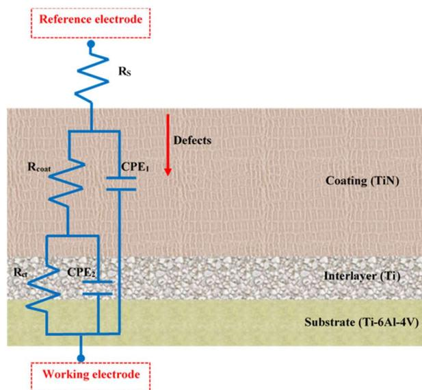
**Fig. 5.** Proposed equivalent electrical circuit for modelling corrosion behaviour of coatings
