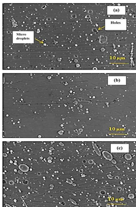
**Fig. 2.** SEM images of TiN coatings deposited at different bias voltages of the substrate: (a) -150 V, (b) -200 V, and (c) -250 V
