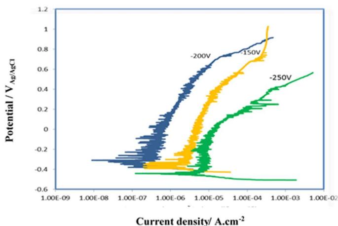
**Fig. 6.** Polarization curves of Ti-6Al-4V samples coated at different bias voltages
