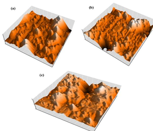
**Fig. 3.** Three-dimensional AFM images of deposited coatings at voltages of: (a) -150 V, (b) -200 V and (c) -250 V
