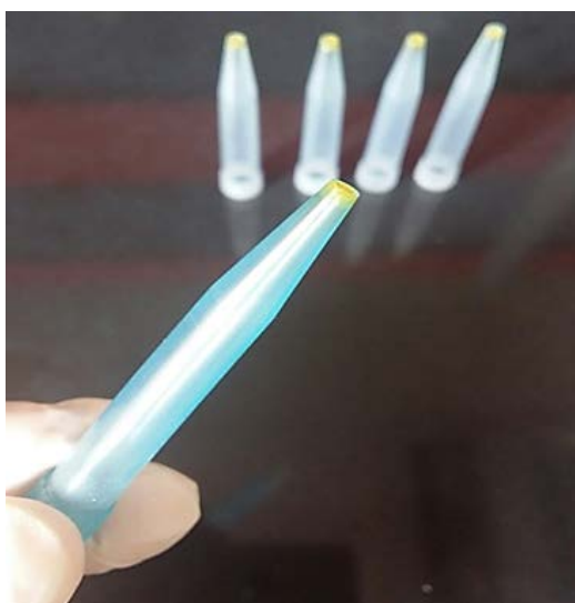
Fig. 1. Image of plastic tube with the PVC membrane
