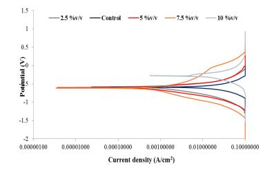
**Fig. 5.** Tafel plots for 304 stainless steel in acidic medium with varied concentrations of natural honey inhibitor
