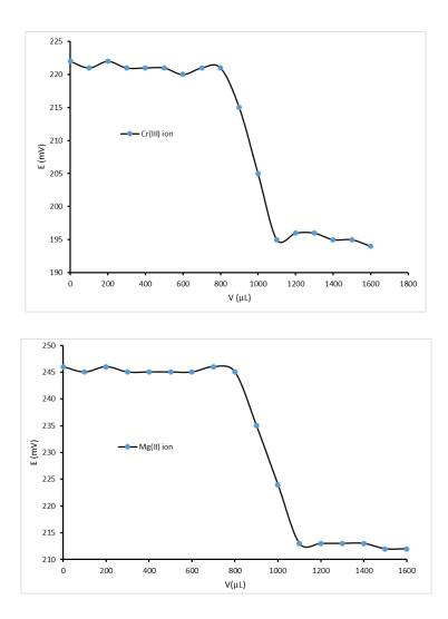
**Fig. 5.** The potentiometric titrations 10.0 mL of  $1.0 \times 10^{-2}$  M of Cr(III) or Mg(II) ions with EDTA solution ( $1.0 \times 10^{-2}$  M)
