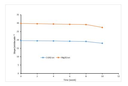
Fig. 4. The lifetimes of the sensors for the determination of Cr(III) and Mg(II) ions
