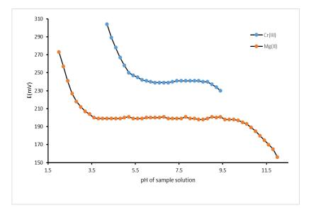
**Fig. 2.** Effect of pH of sample solution on the potential of the Cr(III) and Mg(II) sensors with a concentration of  $1 \times 10^{-3}$  M
