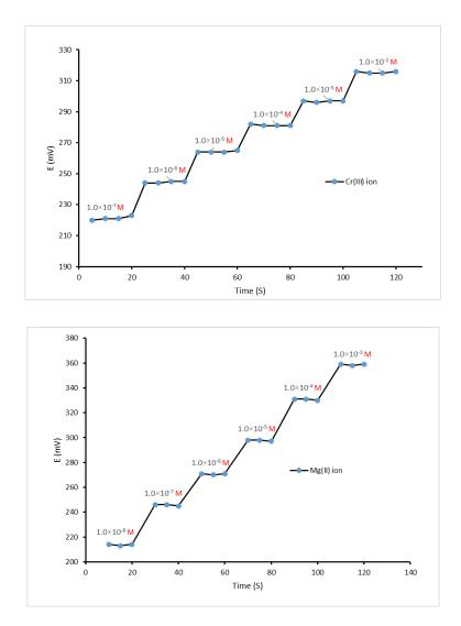
Fig. 3. Response times of the sensors for the determination of Cr(III) and Mg(II) ions
