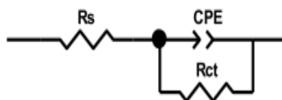
Figure 3. Electrical equivalent circuit showing the progression of the metal/solution interface
