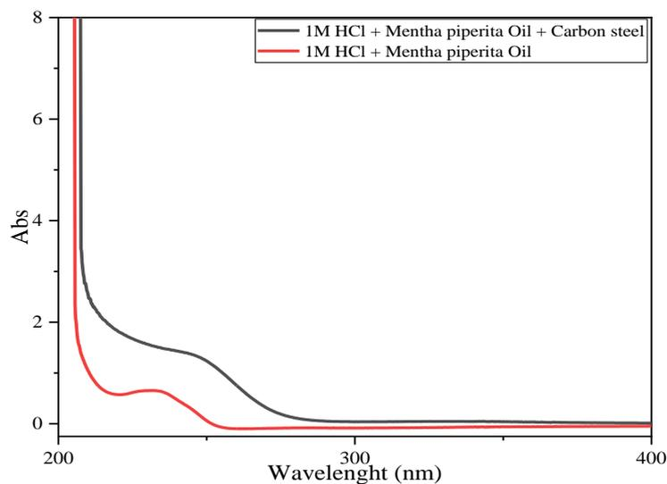
**Figure 9.** UV-visible spectra of the 1 M HCl solution in the presence of *Mentha piperita* essential oil before and after 24 h immersion in carbon steel
