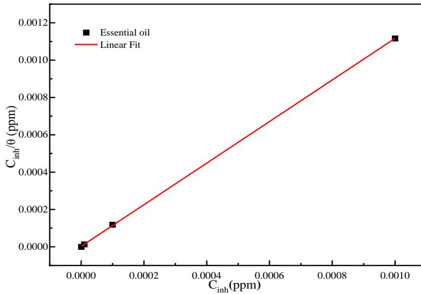
**Figure 5.** Langmuir adsorption of *Mentha piperita* essential oil in a 1 M HCl solution on carbon steel at 303 K
