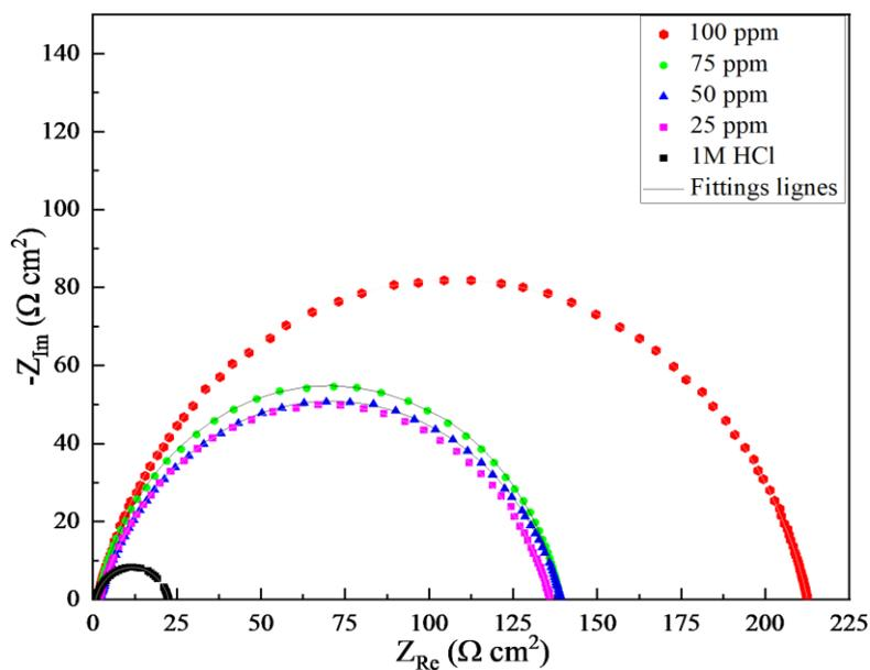
**Figure 2.** Nyquist plots of carbon steel in 1 M HCl containing different concentrations of *Mentha piperita* essential oil at 303 K
