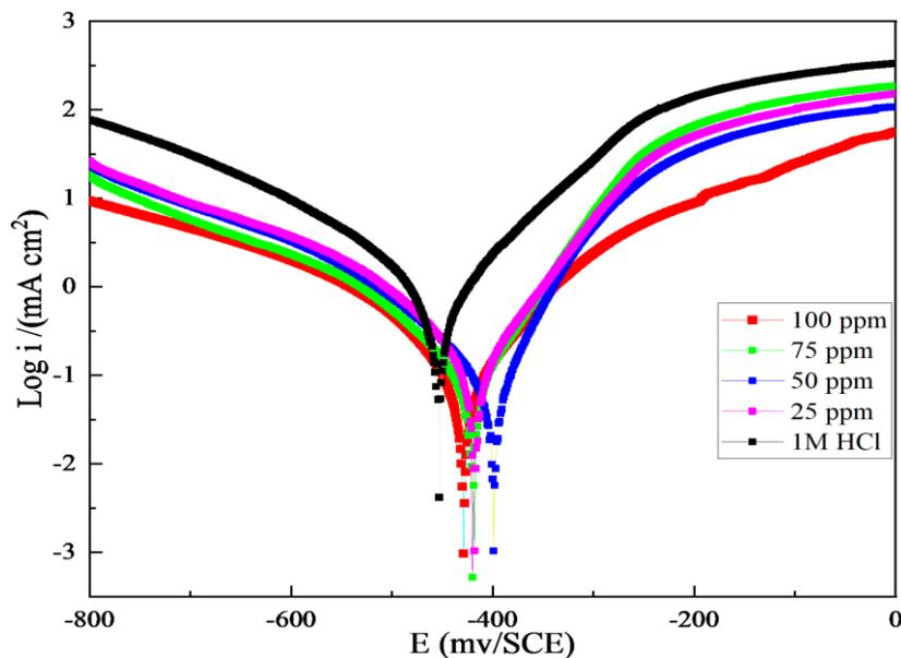
**Figure 1.** Tafel polarization curves for carbon steel at different *Mentha piperita* essential oil concentrations in 1 M HCl at 303K
