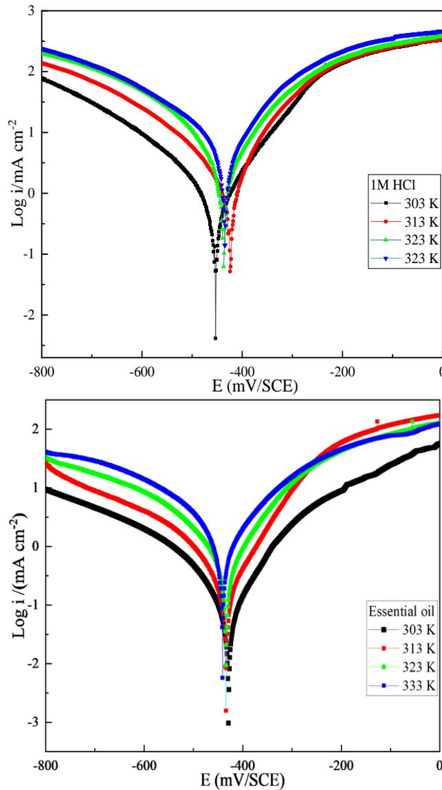
**Figure 6.** PDP curves for carbon steel in 1 M HCl at different temperatures without and with the addition of 100 ppm *Mentha piperita* essential oil
