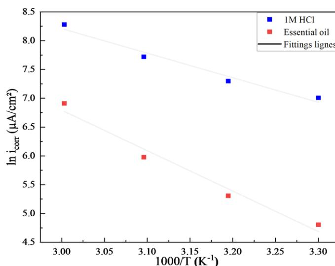
**Figure 7.** Arrhenius lines of carbon steel in 1 M HCl medium in the absence and presence of *Mentha piperita* essential oil
