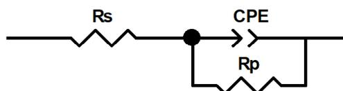
**Figure 4.** Equivalent circuit for EIS data fitting
