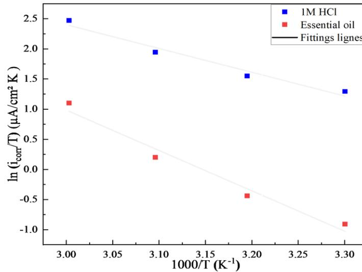
**Figure 8.** Arrhenius lines of  $\ln i_{\text{corr}}/T=f(1/T)$  of carbon steel in 1 M HCl medium in the absence and in the presence of *Mentha piperita* essential oil
