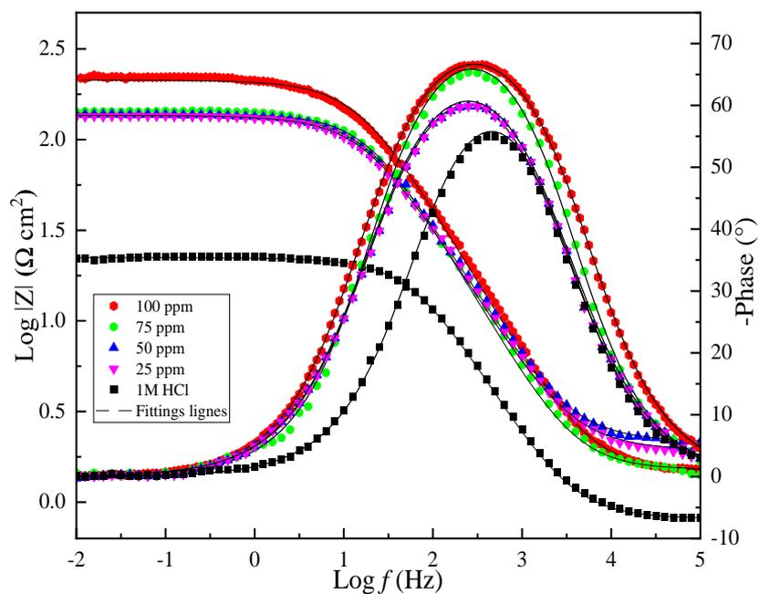
**Figure 3.** Bode graphs for carbon steel at 303 K in 1 M HCl without and with different *Mentha piperita* essential oil concentrations at 303 K
