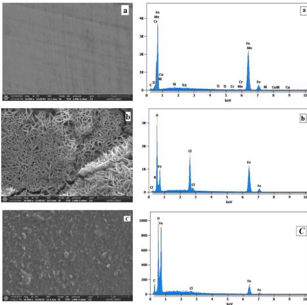
**Figure 10.** SEM/EDS analysis of carbon steel specimens (a) before immersion, (b) after 24 h immersion in 1M HCl and (c) 1M HCl + 100ppm of *Mentha piperita* essential oil at 303 K
